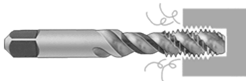
Figure 4 Bottoming-Chamfer Taps for Closed-End Hole Threading
