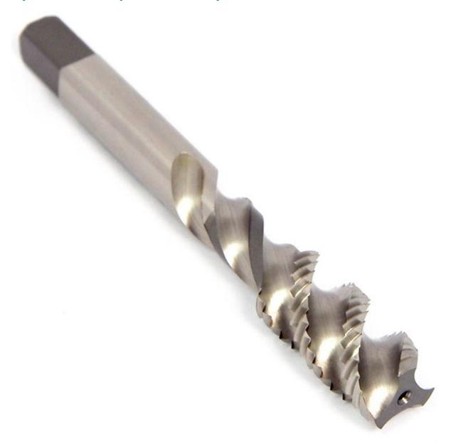
Spiral Flute Taps have an open spiral just like an endmill. Their primary advantage is they eject chips up and out of the hole. They're always preferable over spiral point taps when you have a blind hole.
