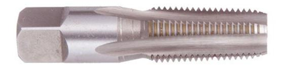
As you might expect, Pipe Taps are the types of thread taps used for tapping pipe threads. There are both straight and tapered pipe taps depending on whether the pipe thread is intended to be straight or tapered. The photo shows a typical NPT Thread Pipe Tap. You can see the taper of the NPT thread profile.
