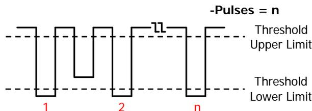
3. **+Edges:** the number of rising edges that rise from below the threshold lower limit to above the threshold upper limit.
