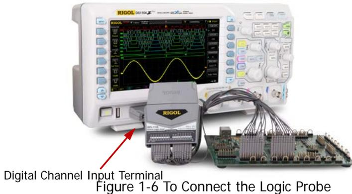
**Note:** The digital channel input terminal does not support hot plugging. Please do not insert or pull out the logic probe when the instrument is in power-on state.
