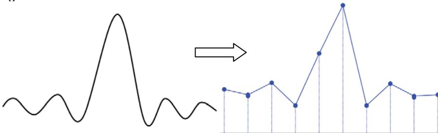
2. **Waveform Confusion:** when the sample rate is lower than twice the actual signal frequency (Nyquist Frequency), the frequency of the waveform rebuilt from the sample data is lower than the actual signal frequency.
