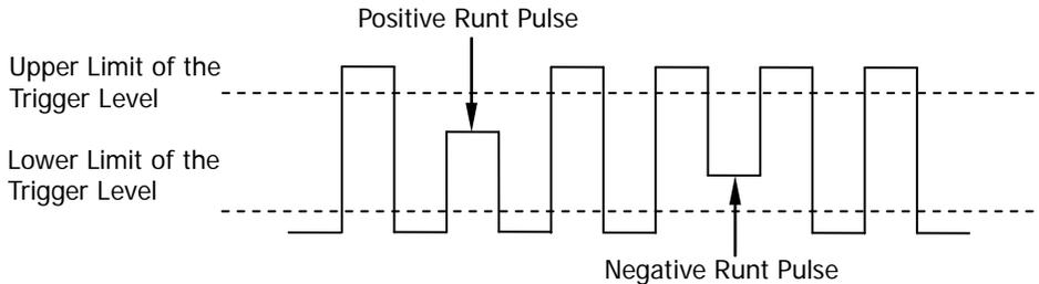
Figure 5-9 Runt Trigger
