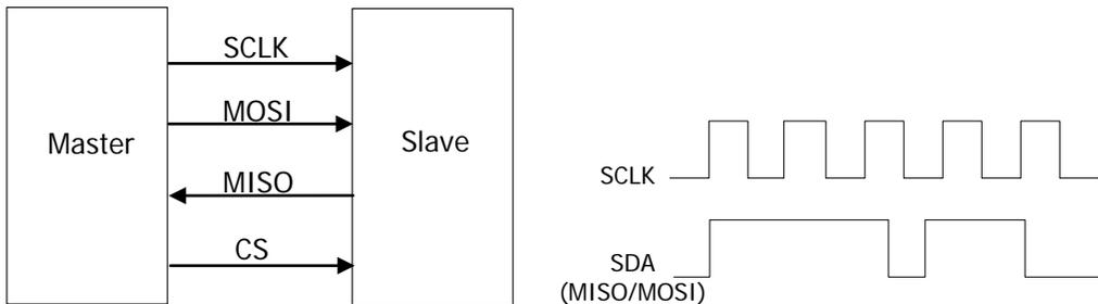
Figure 8-1 SPI Serial Bus
