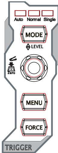
**MODE**: press this key to switch the trigger mode to **Auto**, **Normal** or **Single** and the corresponding state backlight of the current trigger mode would be illuminated.
