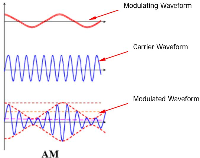
Figure 13-10 Amplitude Modulation
