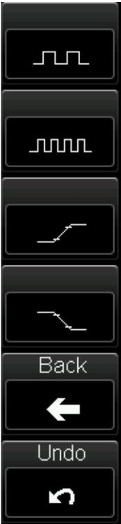
**Single-period:** set the oscilloscope to display single-period signal automatically. Measure the "Period" and "Frequency" of the current signal within a single period and display the measurement results at the bottom of the screen.
