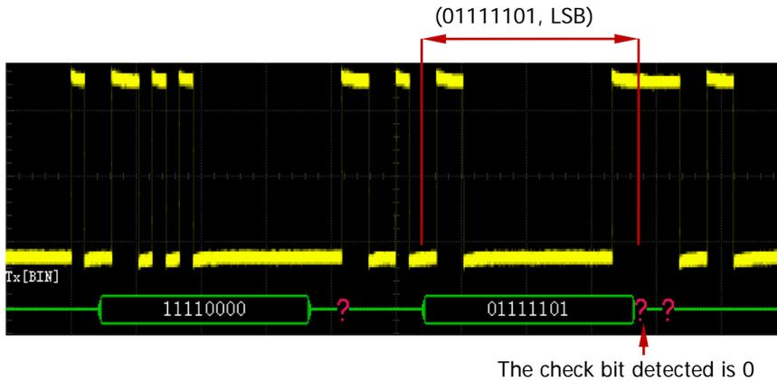
Wherein, there are even number of 1 in the 8-bit data 01111101 and the check bit should be 1; but the check bit detected on the TX is 0, thus check error occurs.
