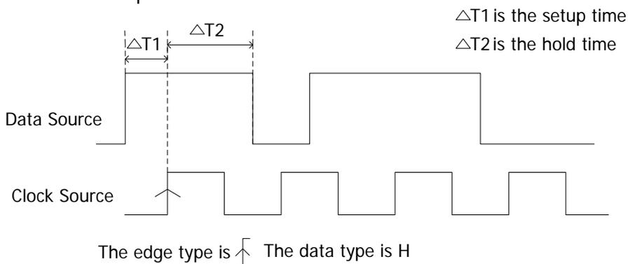
Figure 5-11 Setup/Hold Trigger
