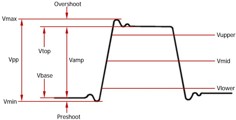
Figure 6-5 Voltage Parameters
