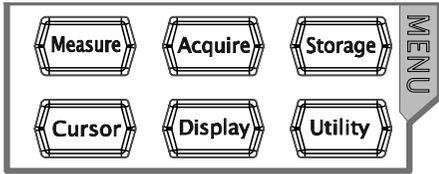
**Measure**: press this key to open the measurement setting menu. You can set the measurement source, turn on or off the frequency counter, all measure, statistic function and etc. Press **MENU** at the left of the screen to open the measurement menus of 37 waveform parameters. Then, press down the corresponding menu softkey to quickly realize one-key measurement and the measurement result will be displayed at the bottom of the screen.
