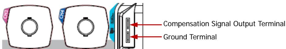
Figure 1-7 To Use the Compensation Signal
