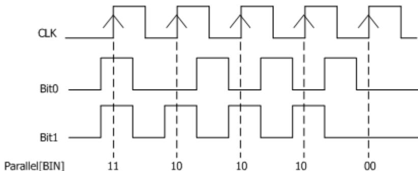
Figure 8-1 Parallel Decoding
