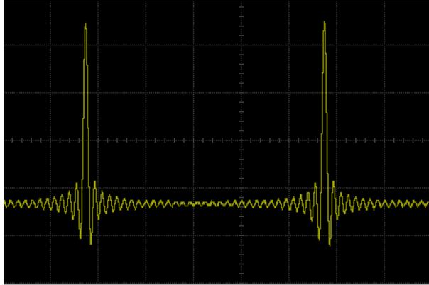
Figure 13-3 Built-in Waveform-Sinc
