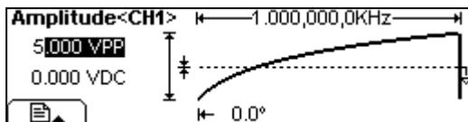
Figure 2-23 Waveform Parameter in the Graph Mode
