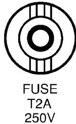
As a fuse, protects the instrument from over-current. Rating: T2A, 250V. For fuse replacement procedure, see page115.
