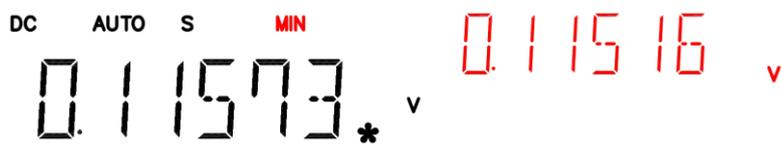
**MIN (MAX)** Indicates Min (Max) measurement
