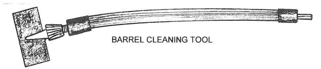
The <u>Abrasive Material Provided</u> is 3M Scotch-Brite Heavy Duty Hand Pad No. 7440. This is 3M's most aggressive hand pad. This product or equivalent is available at most Industrial Hardware Supply Outlets.
