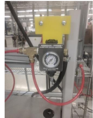
Figure 7 Injection Speed Control
