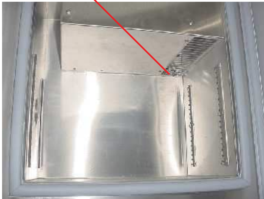
Figure 3. MCB-1.2 Air Temperature Sensor Location
