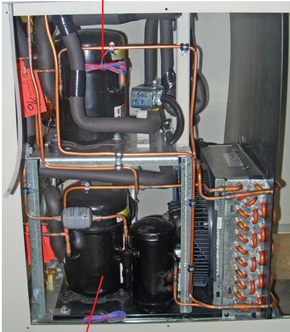
Figure 8. Refrigeration Power Pack MC-3
