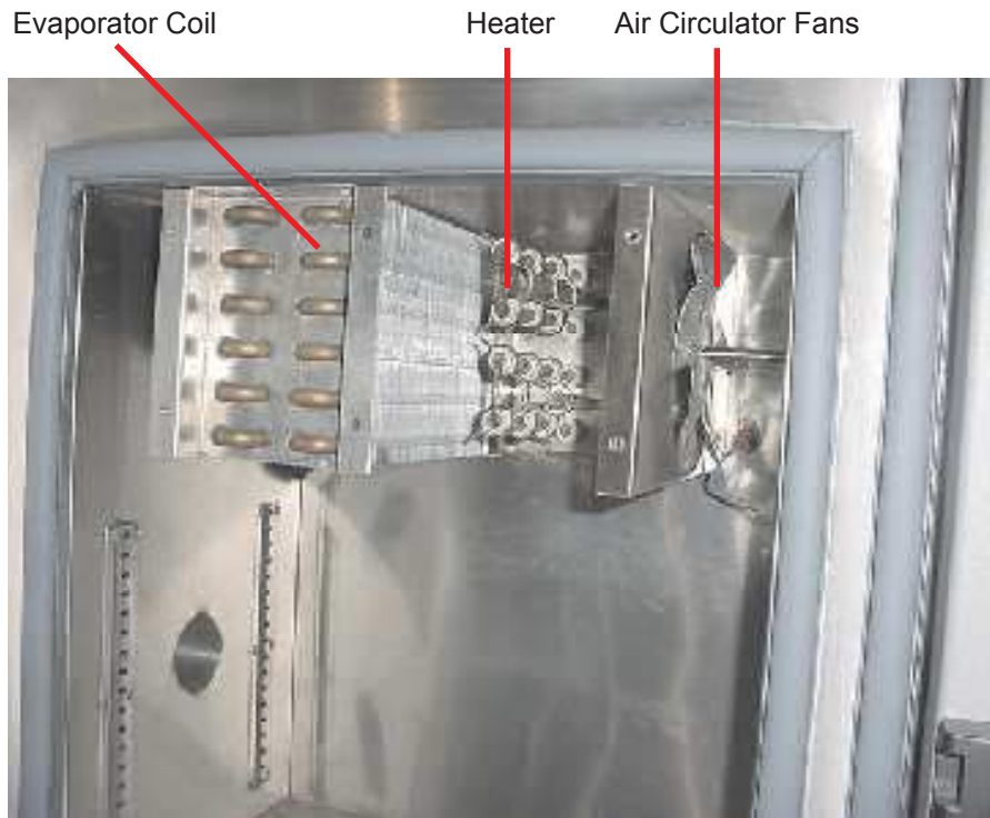
Figure 2. MCB-1.2 Plenum Area
