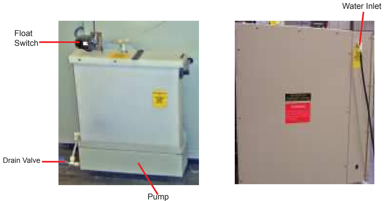
Figure 8. MCB 1.2 Recirculating Water
